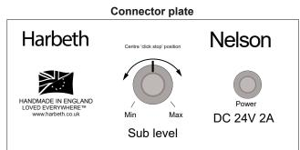
The Nelson connector plate features a sub level control that allows you to adjust the bass (up and down) to suit your music taste and preferences. Please remember that each Nelson is independent, requiring its own separate setup.
